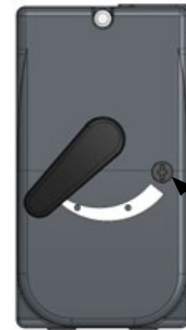
Diversion to the heating circuit. Priority position.
